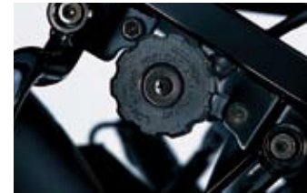
Useful spring preload adjustment
