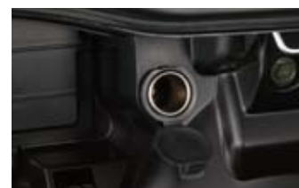
DC power outlet
